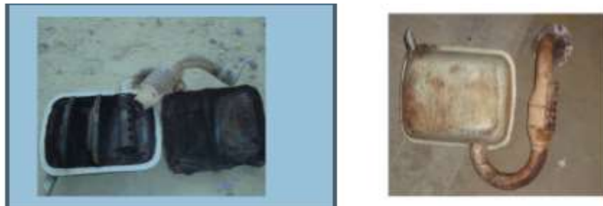
Fig.7.3. Hybrid muffler in cut condition and Hybrid muffler in closed condition
