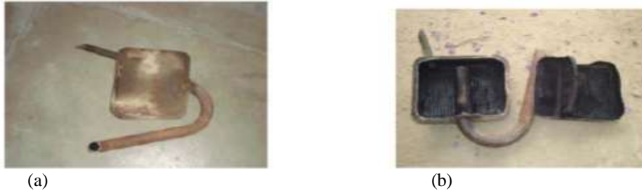
Fig7.1.(a) Reflective muffler in closed condition. (b) Reflective muffler in cut condition
